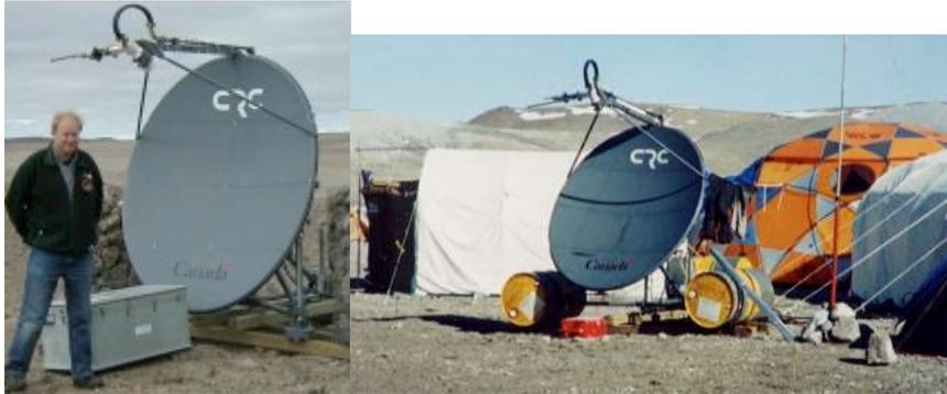
**Figure 1 Conventional 56 kbps C-band data dish used by HMP [10] [5]**
